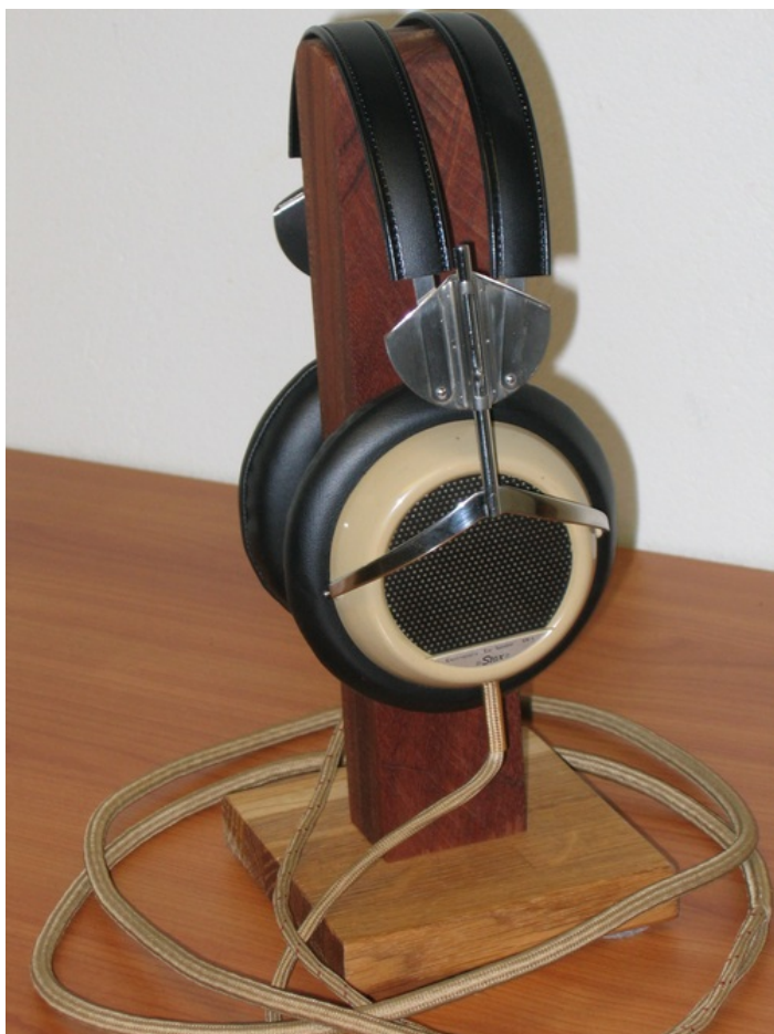
Fig.2. A pair of Stax SR1 Earspeakers. The first ever electrostatic headphones
